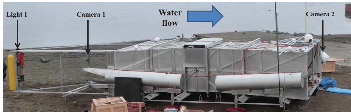
Photo 2. BRI device before deployment, showing mount locations of underwater cameras and light used during deployment in 2014. Water would flow from left to right.
