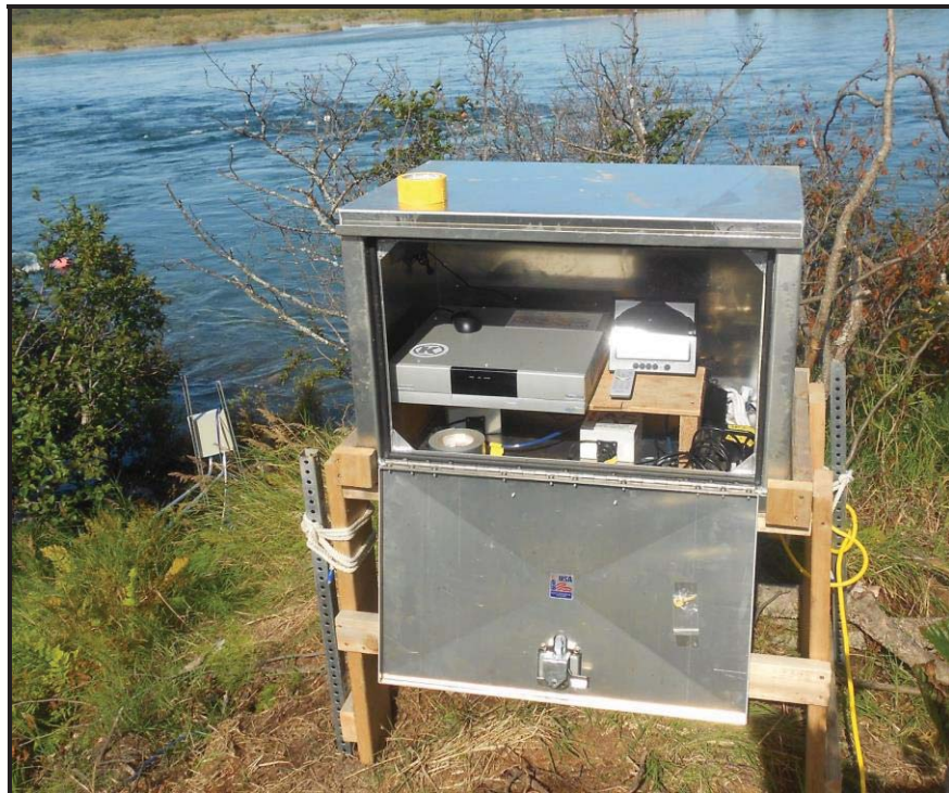
Photo 6. Shoreside cabinetry that housed the video recording system and power link for the BRI RISEC device in 2014. Marker buoys for the submerged device can be seen at top left of photo.
